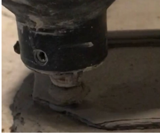
Nozzle digging into print
