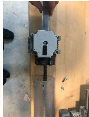
8. Wind/unwind acme screw
