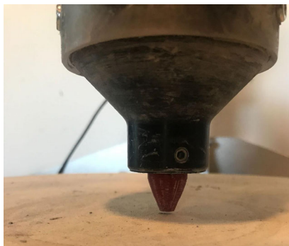
Leave space between nozzle and table
